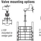
L120/B320 mounted to sluice gate
